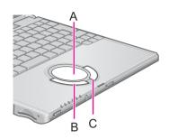
Use the touch pad to move the cursor on the screen and perform computer operations.
